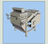
Shear rolls remove the hull and shell from the kernel.
